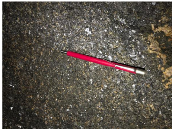
Figure 8. Magnetite ore on the roof of excavated zone in the Mineville Mine. Pencil magnet for scale.
